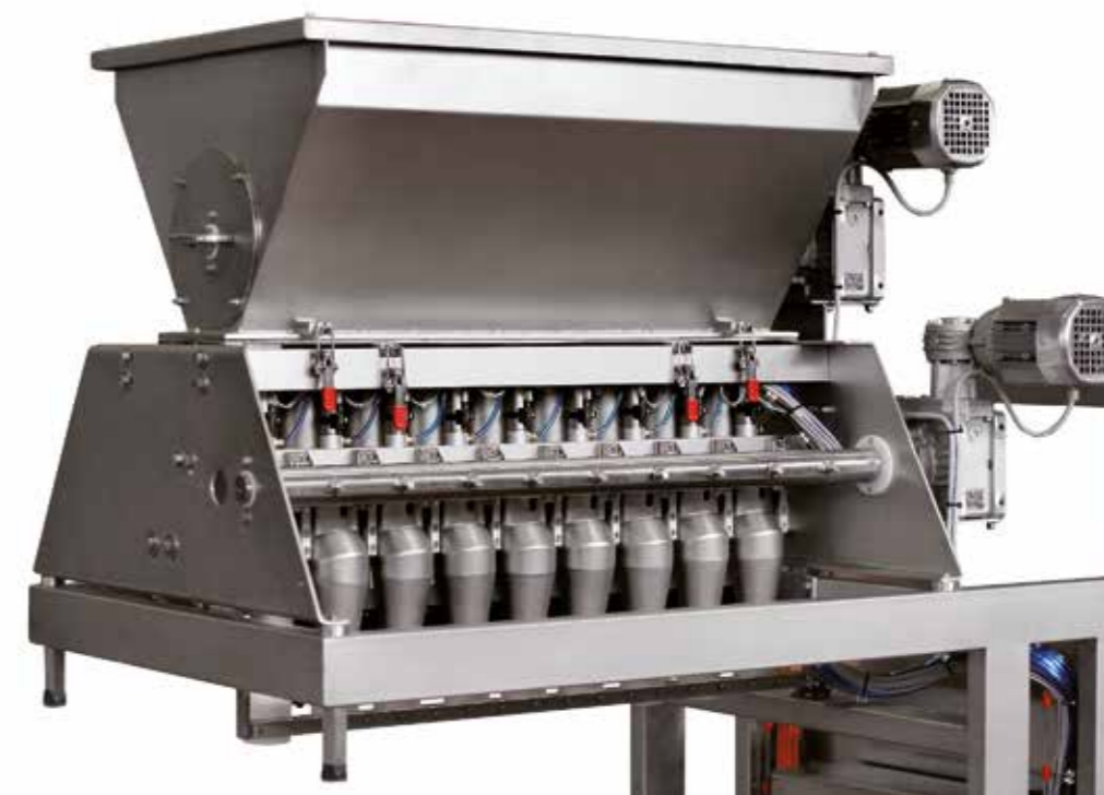
Particulate topping volumetric depositor (chocolate chips, granulated sugar, etc...)
