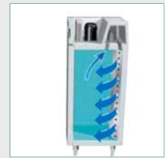
Special ventilation with air-flow conveyors
