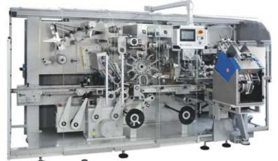
TWO STEP MACHINE FOR WRAPPING CHOCOLATE TABLETS AND BARS, FIRST WITH ALUMINUM WITH HEAT SEAL ON THREE SIDES, SECOND AN EXTERNAL WRAP WITH PAPER OR CARDBOARD CLOSED BY HOT MELT.
