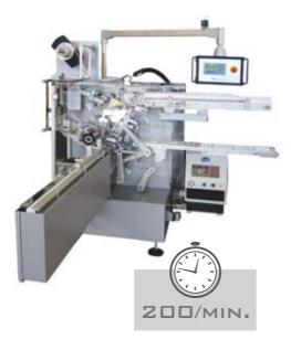
Foil wrapper for flat bottom products. A specific station is provided to glue a shaped cardboard piece on the bottom of the product.
