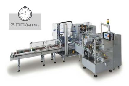
FLEXIBLE MACHINE SUITABLE FOR THE WRAPPING OF FLAT BOTTOM AND SPHERICAL PRODUCTS IN SEVERAL WRAPPING STYLES. THE PRODUCTS ARE LOADED BY ROBOTIC SYSTEM INTO THE MACHINE'S POCKETED IN-FEED BELT.
