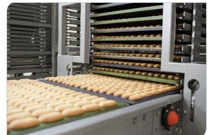
Automated rack loaders/unloaders
