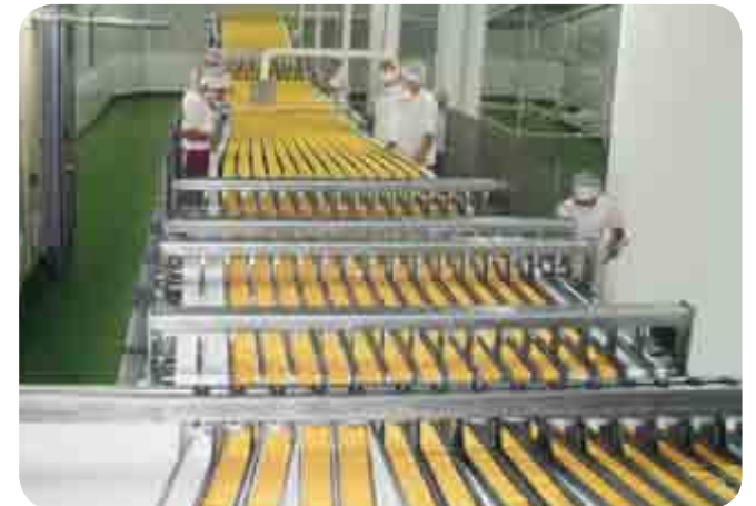
Biscuits on edge are automatically fed to the wrapping machines.
