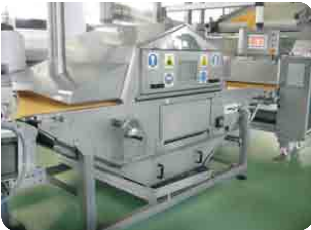
Soda bath unit utilized in the production of snack and pretzel-like products. Two systems can be provided: top sprinkling or full bath.
