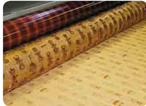
Ink printer installed between the rotary cutter and the scrap pick-up conveyor.
