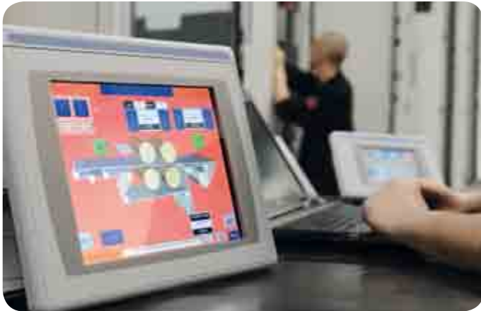
Screenshot of the operator interface which shows the phase-matching between embossing and cutting rolls of the rotary cutter.
