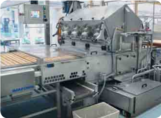
Disk type oil spray machine.
