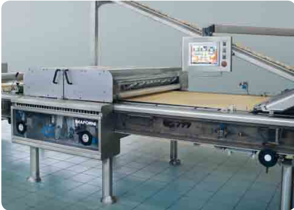
Two rolls rotary cutter unit (one for embossing, the other for cutting). Note the clearance underneath the unit which ensures accessibility for cleaning.
