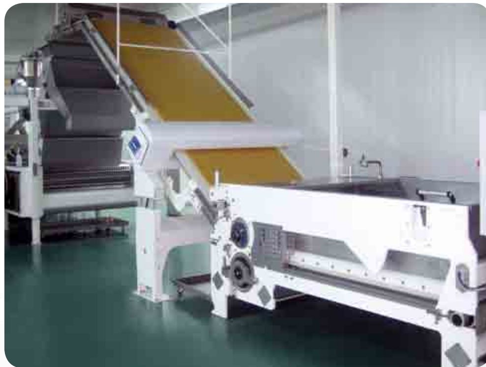
Small footprint dough feeding system suitable for soft and rotary moulded process.
