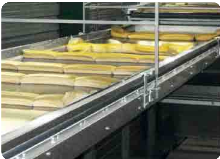
Picture illustrating the principle of operation of the dough portioning system by means of “pocket rolls” . The use of a cutter on the next conveyor can be avoided.
