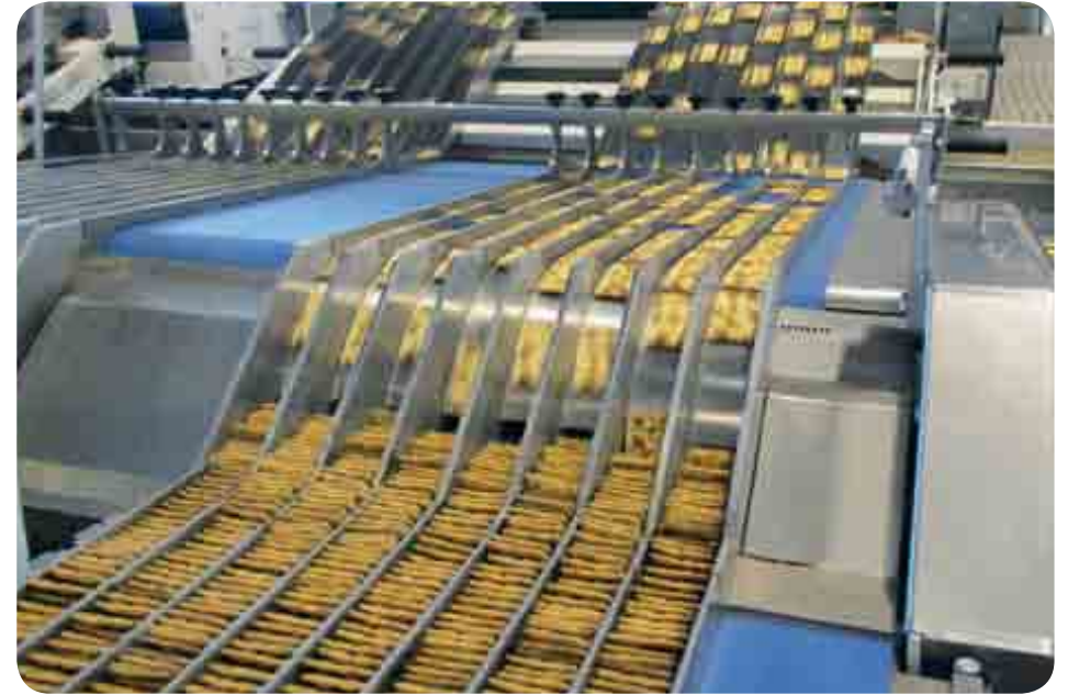
Stainless steel inclined chute to put the crackers between guides, followed by a star-wheel type stacking system.
