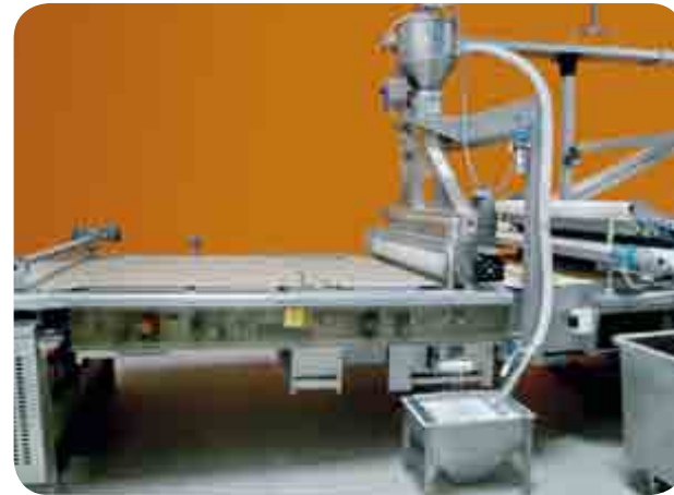
Sugar/salt sprinkler fitted directly on a wire-mesh recovery system. Different recovery systems can be supplied upon request.
