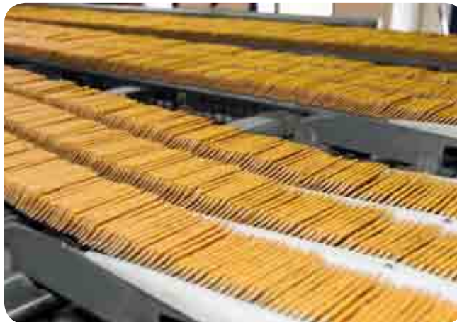
Oscillating guides for stacked soda cracker.
