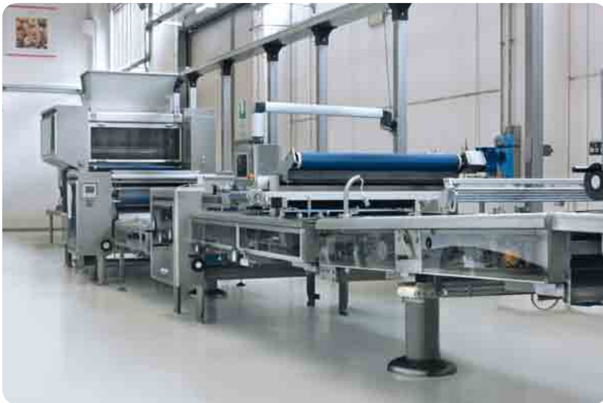
Sheeter and gauge rolls in vertical configuration, followed by rotary cutter/rotary moulder, scraps pick up conveyor and salt/sugar sprinkler unit.
