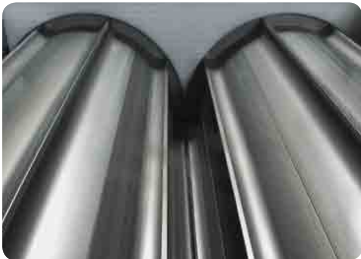
Details of the pocket rollers on the dough feed system.
