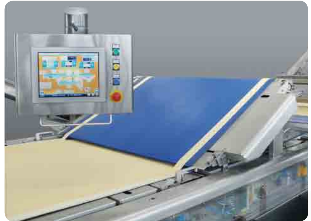
Details of scrap pick-up conveyor and the main control panel of the whole sheeting line.
