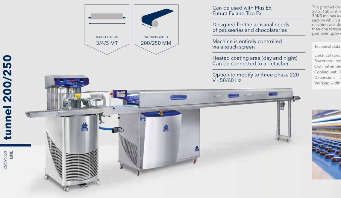
The production speed of this machine ranges from 20 to 150 cm/min. The Tunnel 200/250, length 3/4/5 mt, has a completely integrated coating section which is easily assembled and washed. The machine was designed to allow working with more than one tempering machine, which can be swapped over upon changing the colour of the coating.
